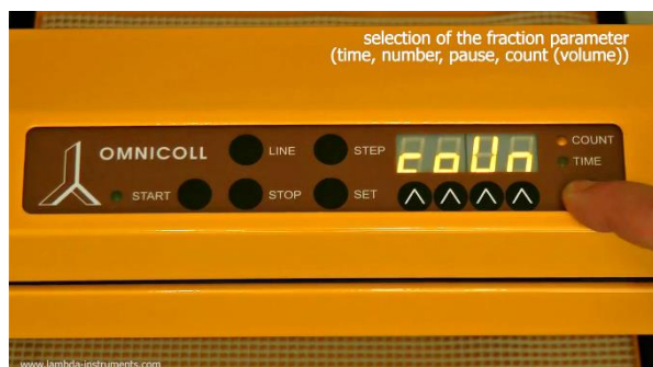
Figure 3.7-4 Selecting parameter COUNT (volume).
