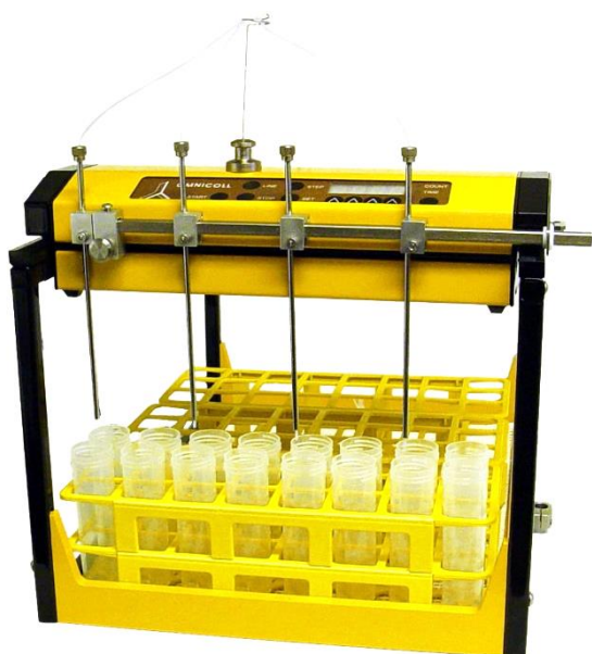
Figure 3.8-1 Example of taking 4x2 fractions in a 4-channel configuration
