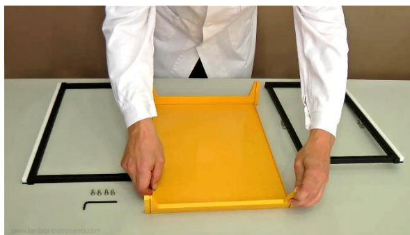
Figure 1.1-2 Push the second tub-sheet into the slots on another shorter side of the yellow support.
