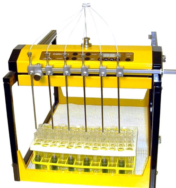
Figure 3.8-2 Example of taking 6x2 fractions in a 6-channel configuration
