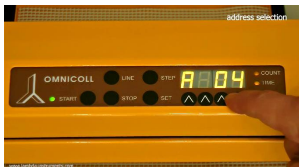
Figure 3.4-16 To change the address press the buttons \wedge \wedge \wedge under the display until the desired number is obtained.
