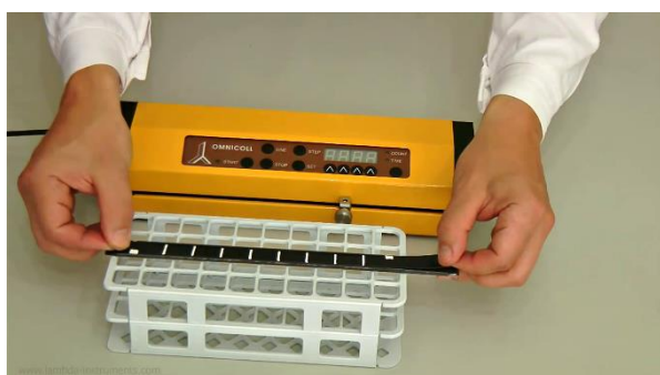
Figure 3.2-3 Place the shorter and broader magnetic coding band into the X-axis holder.
