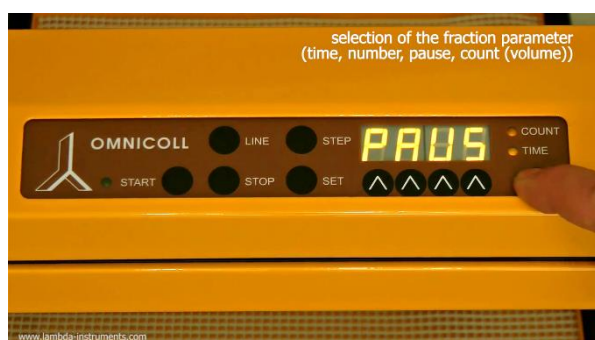
Figure 3.7-6 Selecting the parameter PAUSE for introducing pauses in the program.
