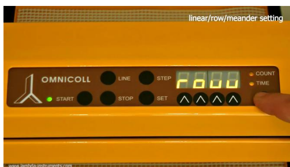
Figure 3.4-2 “row” for row mode of collection appear on the display. Press the SELECTION (below COUNT / TIME) button to select the desired mode of collection.
