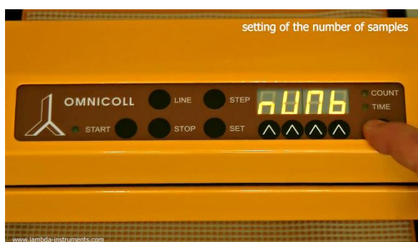
Figure 3.7-7 Selecting the parameter NUMBER for collecting a number of samples.
