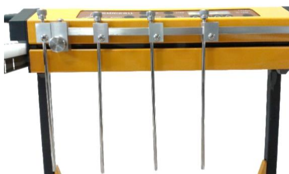
Figure 1.4.1-9 Slide the tubing guide into the tubing guide holder, so that a convenient height above the tubes is obtained. Fix the tubing guide to the holder using the corresponding socket key (hex-key).
