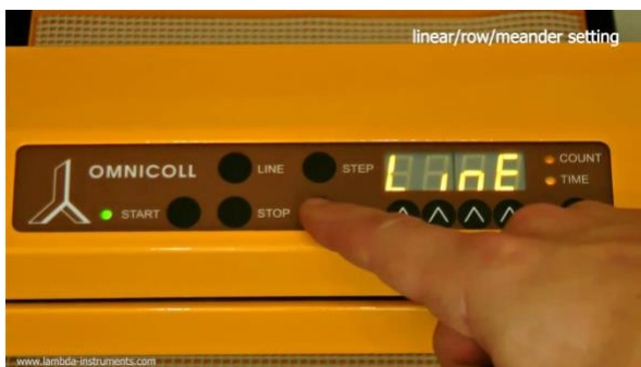
Figure 3.4-5 Confirm the selected mode of collection by pressing SET button
