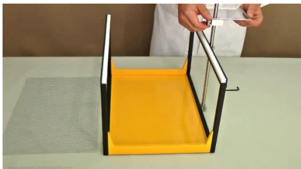
Figure 1.1-7 Push the metal rod through both fixation nuts on the right side of the frame and fasten them with screws. If needed fix the support plate on the metal.
