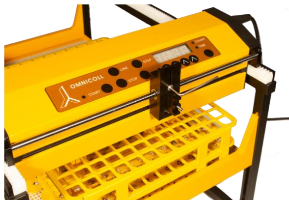
Figure 1.4.2-8 The holder is fixed with one screw using a hexagonal key.
