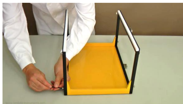
Figure 1.1-6 Tighten it securely with the help of the provided hexagonal key.
