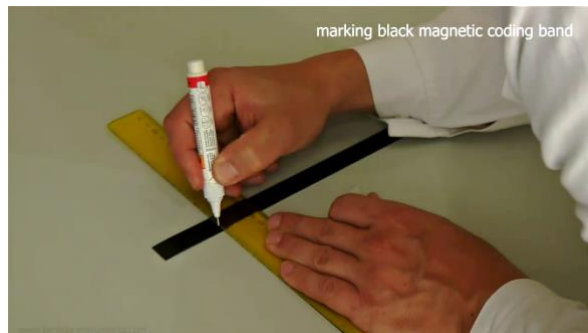
Figure 3.3-2 Draw the white lines correctly on the pre-marked places. Reserve approximately 2cm of the coding band for the beginning and end-position signals.
