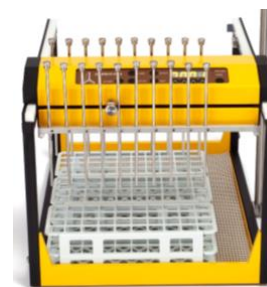
Figure 1.4.1-3 Example of taking 20 simultaneous fractions in a 20-stream (channel) configuration
