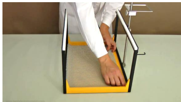
Figure 1.1-8 Place the fixing mat in the support. When needed clean the mat from dust and dirt with a humid cloth. Make sure that the mat is dry before use.
