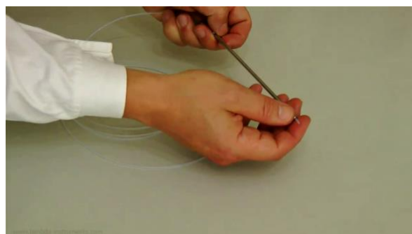
Figure 1.2-4 Push the tubing through the tubing guide and make sure a few mm ( \approx 5\text{mm} ) of PTFE tubing reach out of the tubing guide so that the drops form only at the tip of PTFE tubing.
