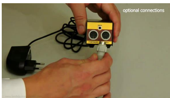
Figure 1.5-5 Connect the OMNICOLL fraction collector to the "OMNICOLL" socket in the communication module.
