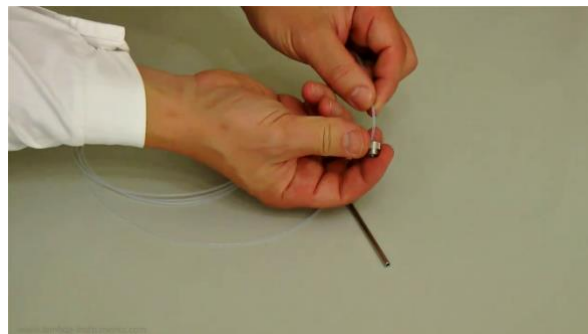
Figure 1.2-2 Push the delivered PTFE tubing through the pipe guide as shown.
