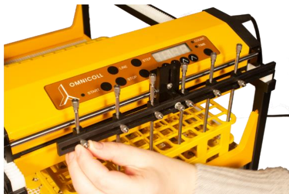
Figure 1.4.2-12 The tube guide is fixed with one bolt.
