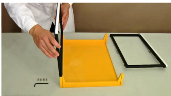
Figure 1.1-3 Insert the black frame into the corresponding slots of the yellow supports
