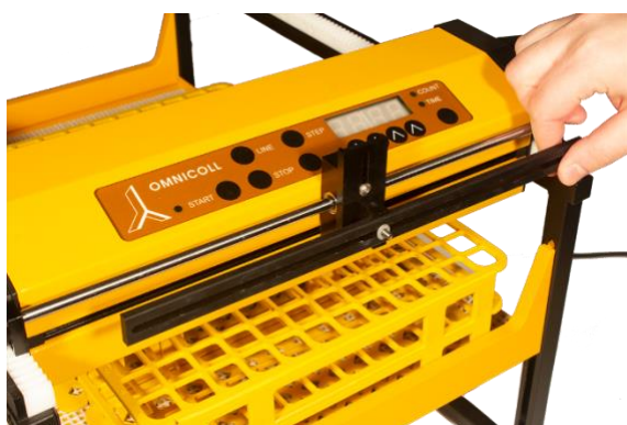
Figure 1.4.2-9 The moving arm is mounted on the holder.
