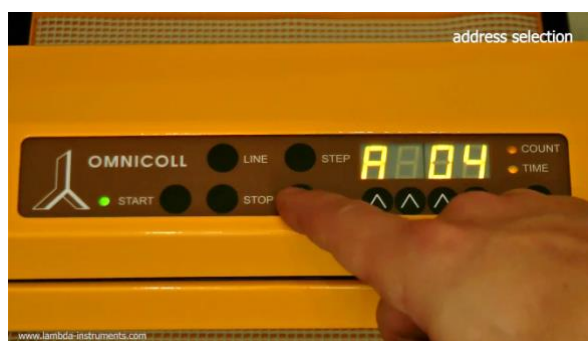
Figure 3.4-17 Confirm the choice by pressing the button SET
