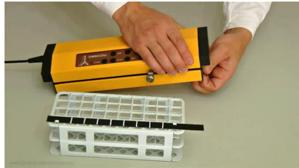
Figure 3.2-2 Pull the X-axis coding band holder from the OMNICOLL control unit as shown.
