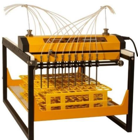
Figure 1.4.2-1 Front side of the customized multi-channel fraction collector LAMBDA OMNICOLL for 18 streams . (Accessory for fixed multi-stream collection adjustable up to 64 channels art. no. 6952).
