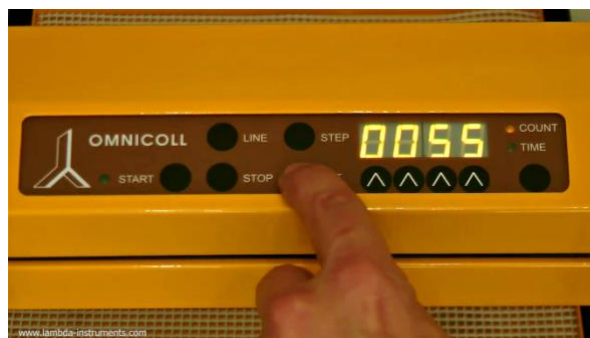
Figure 3.6-4 Confirm the selection by pressing the SET button.
