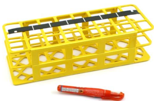
Figure 3.1-3 The beginning and the end of a row are indicated by short lines (about half the length of the normal stripes or less and ~5 mm broad) made on the lower edge (for the beginning) and upper edge (for the end) of the coding band, respectively.
