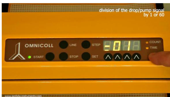
Figure 3.4-12 By pressing the COUNT/TIME button select the desired division factor.
