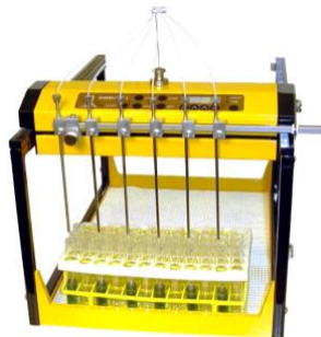
Figure 1.4.1-2 Example of taking 6x2 fractions in a 6-channel configuration
