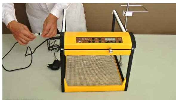
Figure 1.1-10 Connect the cable of the control unit of the LAMBDA OMNICOLL fraction collector and sampler with the cable of the power supply plug.
