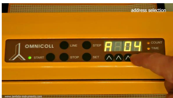
Figure 3.4-16 To change the address press the buttons ^ ^ ^ ^ under the display until the desired number is obtained.
