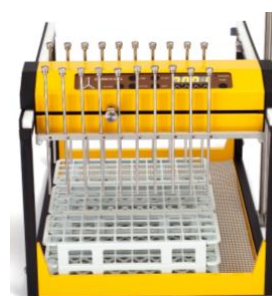
Figure 1.4.1-3 Example of taking 20 simultaneous fractions in a 20-stream (channel) configuration
