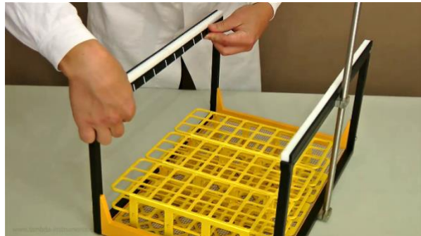
Figure 3.3-6 Place the coding band on the left internal side of the metal frame just under the gear bar.
