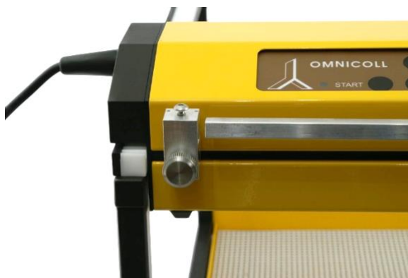
Figure 1.4.1-5 Place the bar holder on the tubing guide holder screw.
