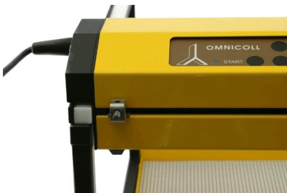
Figure 1.4.1-4 Unscrew the tubing guide holder screw on the moving arm of the LAMBDA OMNICOLL fraction collector
