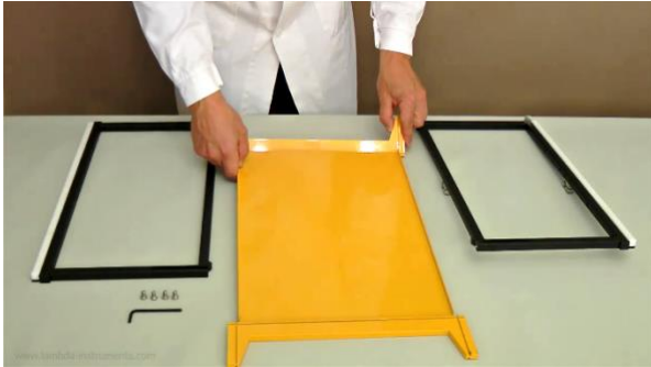
Figure 1.1-1 Push the first tub-sheet into the slots on one of the shorter sides of the yellow support.
