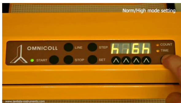
Figure 3.7-2 Use the COUNT/TIME button to select the “ high ” mode.
