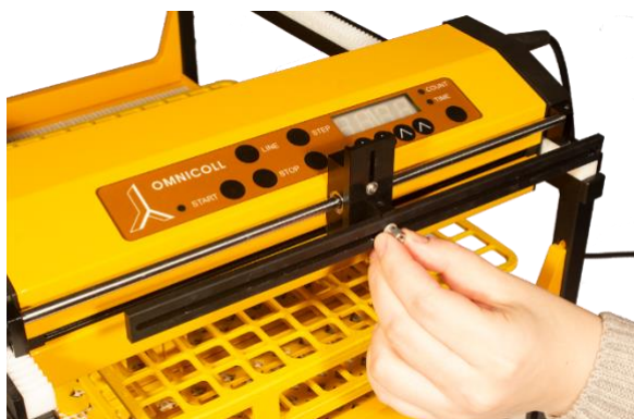
Figure 1.4.2-10 The moving arm is fixed with one washer and bolt.
