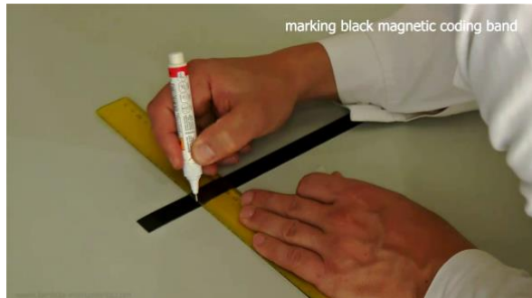
Figure 3.3-2 Draw the white lines correctly on the pre-marked places. Reserve approximately 2cm of the coding band for the beginning and end-position signals.
