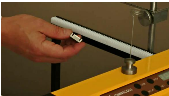
Figure 1.1-11 Place the supplied magnet on the right inner side of the frame to stop the fraction collection.
