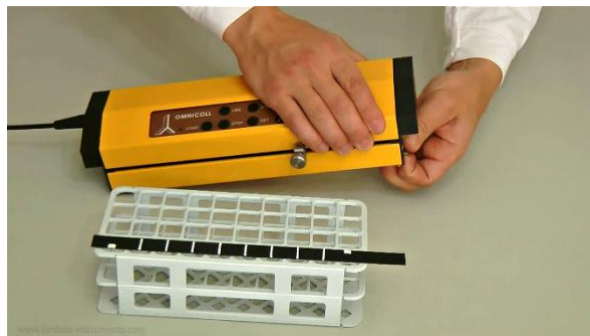
Figure 3.2-2 Pull the X-axis coding band holder from the LAMBDA OMNICOLL control unit as shown.
