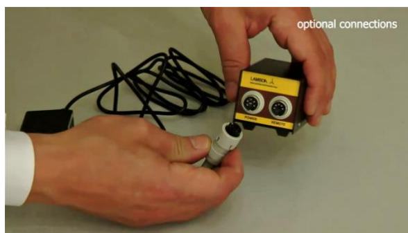
Figure 1.5-4 Connect the power supply to the “POWER” socket in the communication module.
