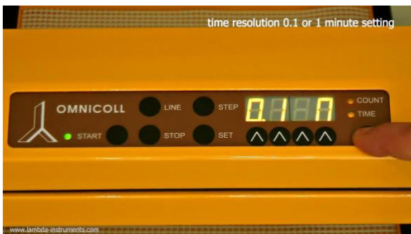
Figure 3.4-8 By pressing the button COUNT / TIME below the COUNT and TIME LEDs you can select to use 0.1 minute steps " 0.1M " or 1 minute steps " 1M ".
