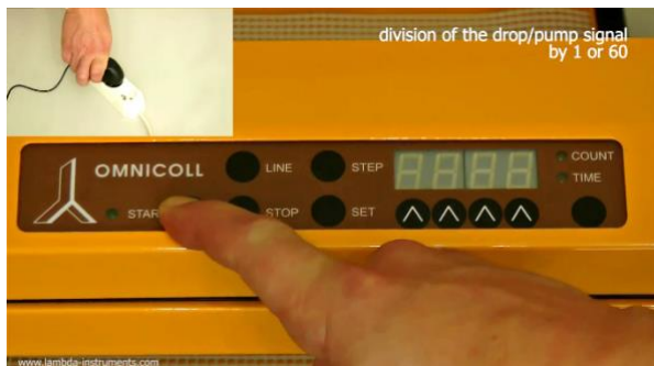
Figure 3.4-10 Press the button START while plugging the power supply into the mains.
