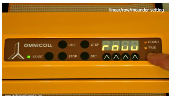
Figure 3.4-2 “ rouu ” for row mode of collection appear on the display. Press the SELECTION (below COUNT / TIME) button to select the desired mode of collection.
