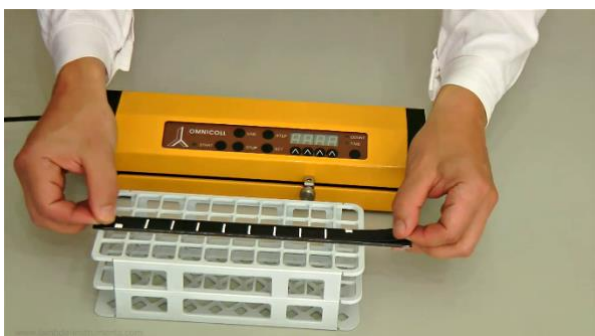
Figure 3.2-3 Place the shorter and broader magnetic coding band into the X-axis holder.
