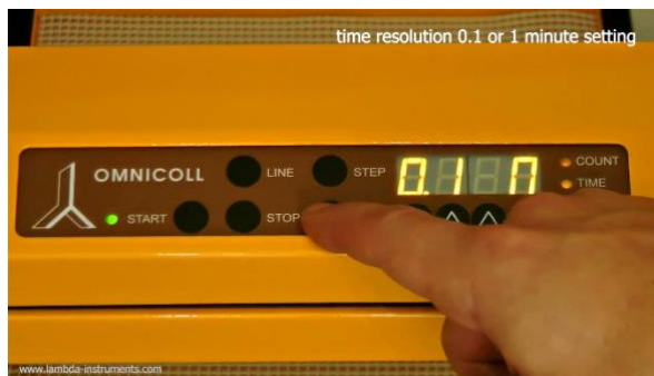
Figure 3.4-9 Confirm the choice by pressing the button SET .
