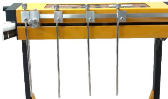
Figure 1.4.1-9 Slide the tubing guide into the tubing guide holder, so that a convenient height above the tubes is obtained. Fix the tubing guide to the holder using the corresponding socket key (hex-key).
