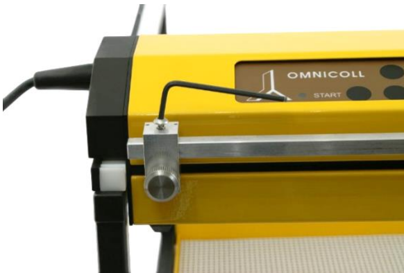
Figure 1.4.1-8 Screw the bar holder on the moving arm of the fraction collector with the corresponding socket key (hex-key). Use e.g., a thin spatula to push the screw through the moving arm.
