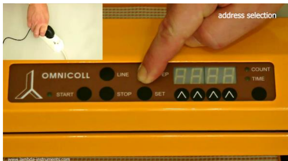
Figure 3.4-14 While keeping the direction button STEP pressed connect the fraction collector to the mains.
