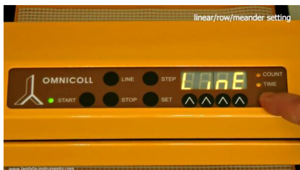
Figure 3.4-4 “ Line ” for linear mode of collection appear on the display.
