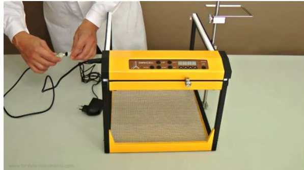
Figure 1.1-10 Connect the cable of the control unit of the LAMBDA OMNICOLL fraction collector and autosampler with the cable of the power supply plug.
