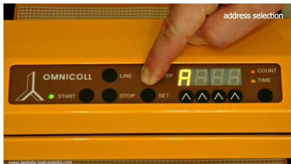
Figure 3.4-15 The message "A" and two numbers will appear on the display. This number from 00 to 99 is the current address of the fraction collector.
