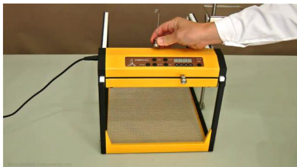
Figure 1.2-1 Place the magnetic tubing holder conveniently in the centre of the fraction collector carriage and control unit.
