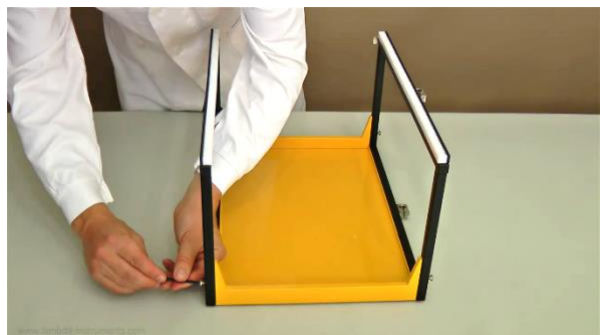
Figure 1.1-6 Tighten it securely with the help of the provided hexagonal key.
