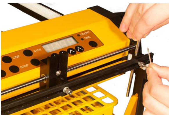
Figure 1.4.2-13 The tube guide can be raised or lowered with a hexagonal key.
