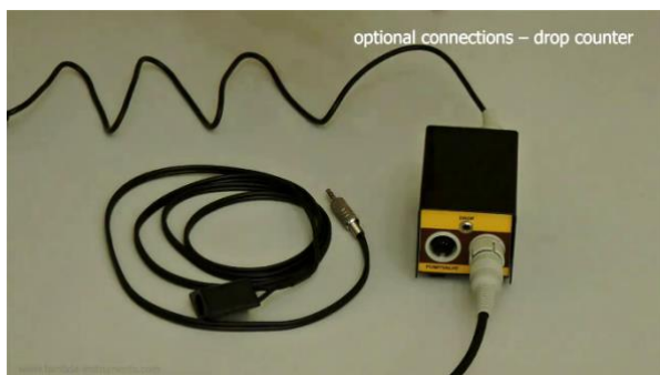
Figure 1.5-1 Showing drop counter (detector) cable with the communication module (Art. No.: 6929)
