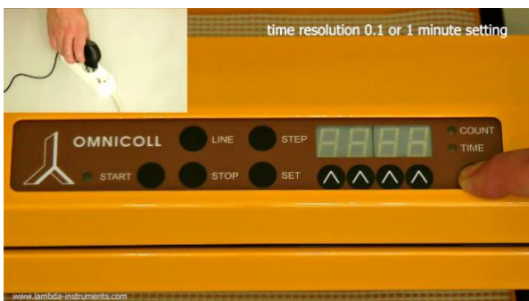
Figure 3.4-6 Press the button COUNT/TIME while connecting the power supply to the mains.
