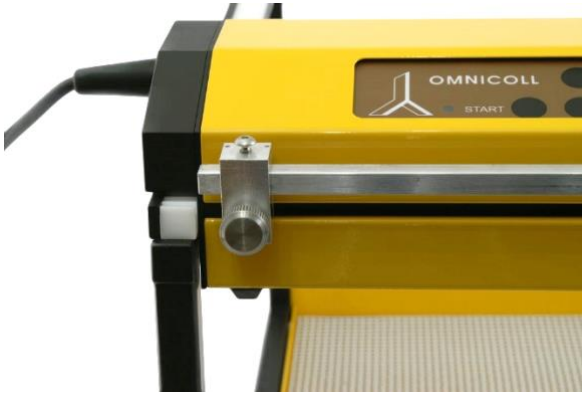
Figure 1.4.1-6 Insert the rectangular bar into the bar holder as shown.
