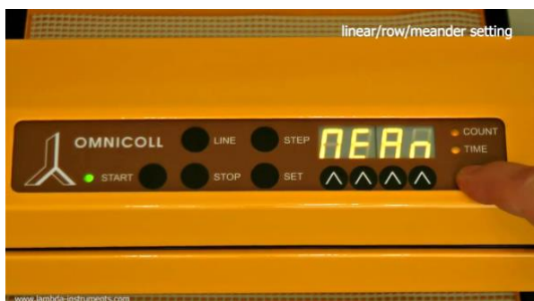
Figure 3.4-3 “ Mean ” for meander-like mode of collection appear on the display.
