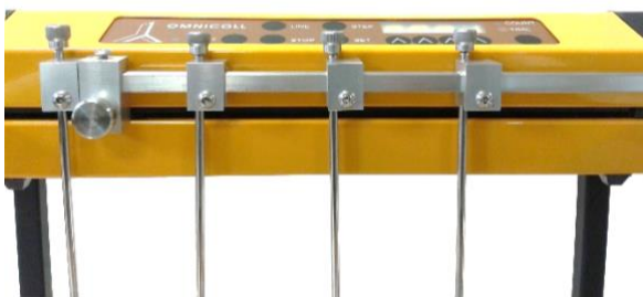
Figure 1.4.1-10 Place the tubing guide holder at the desired fraction position and secure it with the socket head screw using the corresponding socket key (Allen key).
