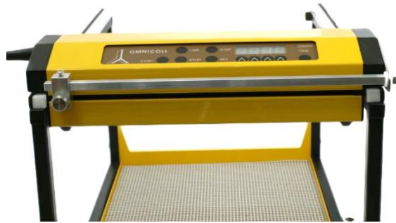
Figure 1.4.1-7 Slide the right end of the bar through the opening on the guide plate.
