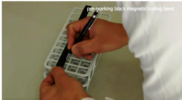
Figure 3.3-1 Place the coding bands on the tube rack and mark the fractioning position with a normal pencil.
