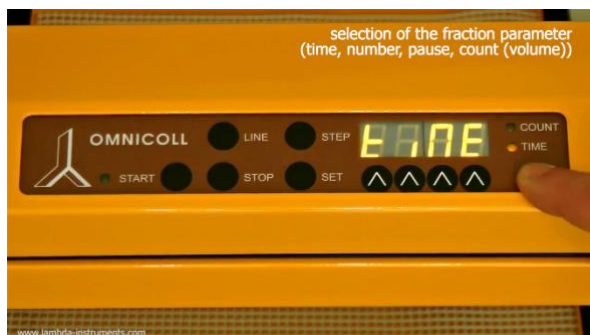
Figure 3.7-5 Selecting the parameter TIME to perform the program for a desired time.
