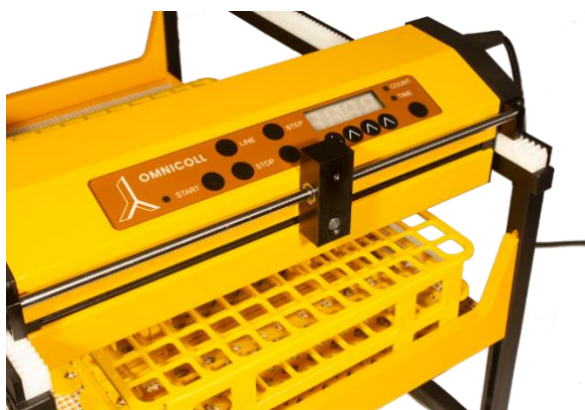
Figure 1.4.2-7 The moving arm holder attaches to the black rectangle attached to the device.
