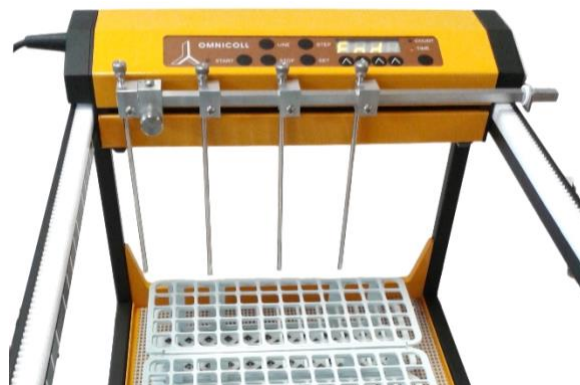
Figure 1.4.1-11 Place the tubing guide holder in position above the first fraction of each stream (channel). If 4 streams are collected in a row, the place: first tubing guide over tube no. 1, second tubing guide over tube no. 4, third tubing guide over tube no. 7 and fourth tubing guide over tube no. 10
