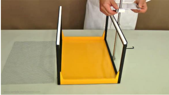
Figure 1.1-7 Push the metal rod through both fixation nuts on the right side of the frame and fasten them with screws. If needed fix the support plate on the metal.
