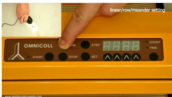
Figure 3.4-1 Press the button LINE continuously while plugging the power supply into the mains.
